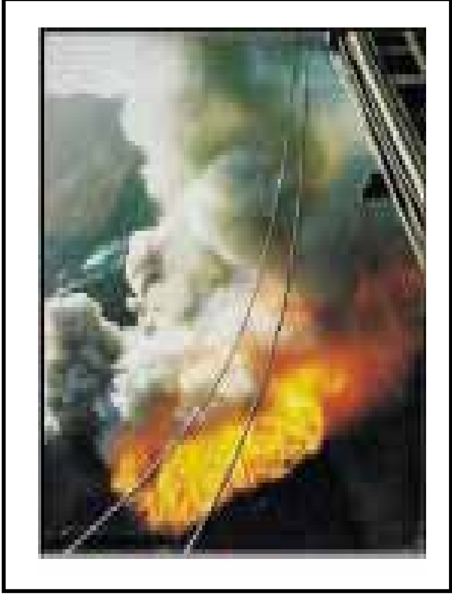
Figure 8 Coal fire explosions in the dragline bucket while loading out burning coal
